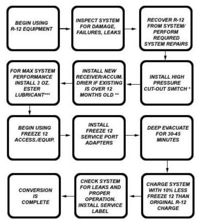
NOT REQUIRED IF A/C SYSTEM NOT EQUIPPED WITH HIGH PRESSURE RELIEF VALVE
